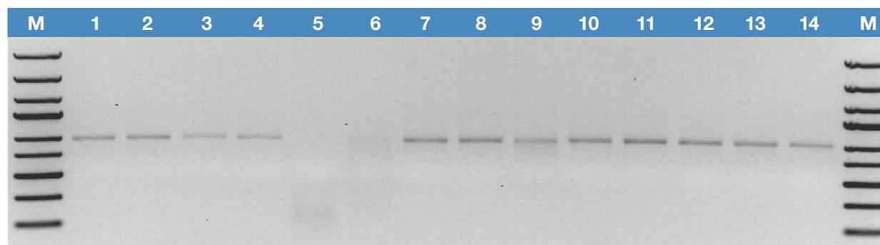
Figure 2: Ribonucleases Assay: Electrophoresis gel with 1% agarose buffer and ethidium bromide stain. M: GeneRuler™ Express DNA Ladder; Lanes 1,2: Negative control; Lanes 3, 4: 30 ng/15 µL RNA transcript control; Lanes 5, 6: Smart2Pure 60 L reservoir water; Lanes 7, 8: Pre-challenge water; Lanes 9, 10: 2.5 L post challenge; Lanes 11, 12: 5 L post challenge; Lanes 13, 14: 10 L post challenge. Sample is considered have RNase activity if degradation of RNA is observed.
